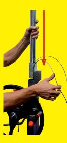
and tighten the nut on the axis with a 17 mm (11/16") flat wrench and an 8 mm (5/16") hex wrench.
