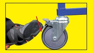
Push the brake lever while lifting the safety brake latch, to lower the top rack. If you have to lower the top rack loaded, pay attention to control the descent by pushing slightly on the main brake lever. In case of a main brake default, release immediately the safety brake lever in order to stop the descent right away.
