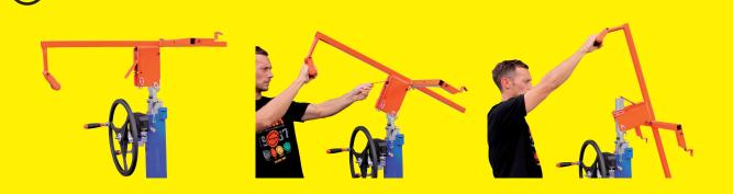
Insert the arms in the tube according to the selected setting, the retractable pin must be locked in the hole.
