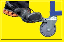
Once the board touches the ceiling, position the board perfectly and lock the wheel brakes while screwing the board.
